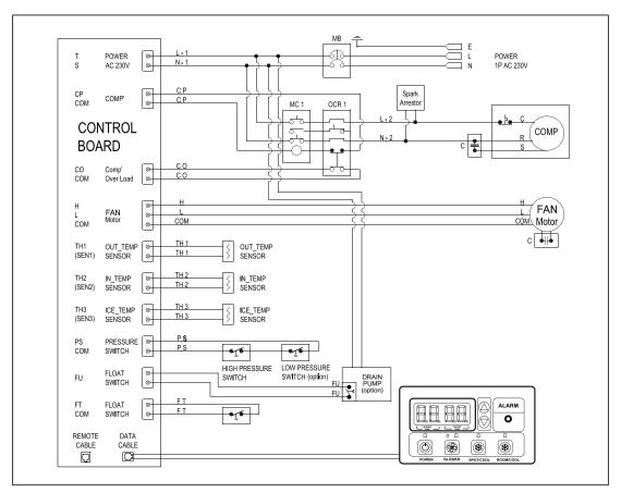
Figure 13 - Circuit Wiring Diagram (WPC 168 / WPC 208)
