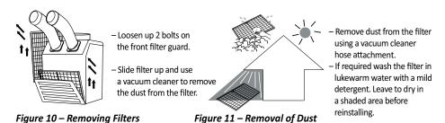
WARNING! Do not operate without the filter fitted.
