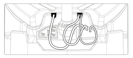
Route the **fan head power cord, atomizer drain hose, and water inlet hose** through the openings in the back of the **water tank** as shown above.
