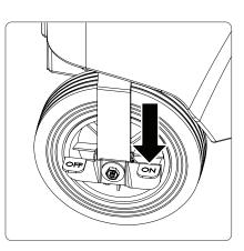
Before you get started, be sure to lock both of the **rear wheels** by pressing down on the brake lever to set them to the **ON** position.
