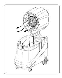
Once installed, the **atomizer** (metal disk) will be facing the **water tank**, air will be blown over the **water tank** when the Power Breezer is turned on.
