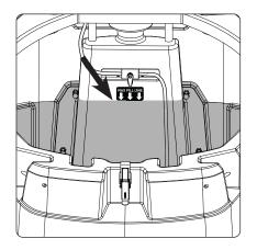
Do not fill the **water tank** above the **max fill level**, as shown. If **water tank** is filled past this level, water may leak out of the **water tank** and cause a hazard around the Power Breezer.
