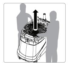
Finish opening the **lid latch** by pulling the upper portion of the latch forward and away from the lid.
