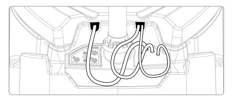
• Route the **fan head power cord, atomizer drain hose, and water inlet hose** through the openings in the back of the **water tank** as shown above.
