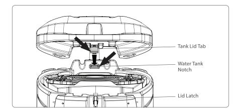
Note the lid tab on the back underside of the lid.
