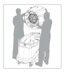
Lift the **fan head** straight up and off the **head support pole.**
