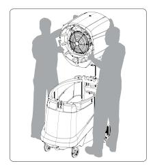
Lift the **fan head** straight up and out of the **water tank**. Carefully rest it on the **edge of the water tank**.
