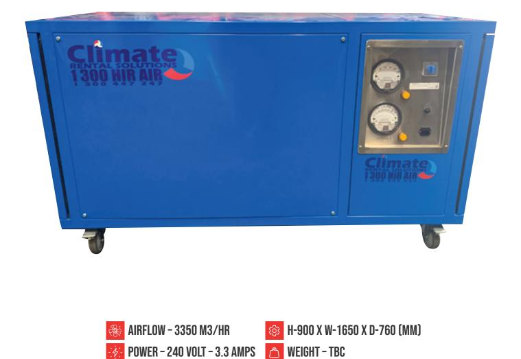
The AFD3350 Air Scrubber is a large portablehigh performance air purifier designed and made in Australia. It delivers a huge3350 m3/hr of HEPA filtered air while drawing less than 4 amps of power. It has a H13 filter but also has the option of a H14 filter.
