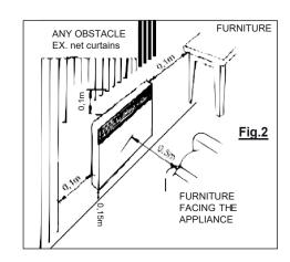
For maximum efficiency, this heater is to be wall mounted between a minimum height of 100mm and a maximum height of 150mm off the floor. This is to allow the necessary volume of air to flow freely through the vents. It is also important to allow a minimum of 100mm clearance at the top and sides of the heater and 500mm from the front (Fig. 2) so as not to force the air back into the heater and activate the Over Temperature Safety Thermal Cut-Out Switch.
