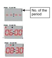
Press the **OK Prog** button to confirm. Period 2 settings are now displayed. Repeat the above steps for Period 3 to set the times that the heater is to turn **ON** and return to **STANDBY**.
