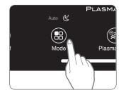
**NOTE:** When in Auto mode the fan speed is automatically adjusted according to the indoor air quality. As the indoor air quality improves, the fan speed will automatically be reduced. If the indoor air quality decreases, the fan speed will automatically increase.
