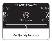
**NOTE**: Air quality level is displayed on the indicator, based on the Particle Sensors. Depending on the immediate environment, the indicator may change frequently in color or stay the same for lengthy periods of time.
