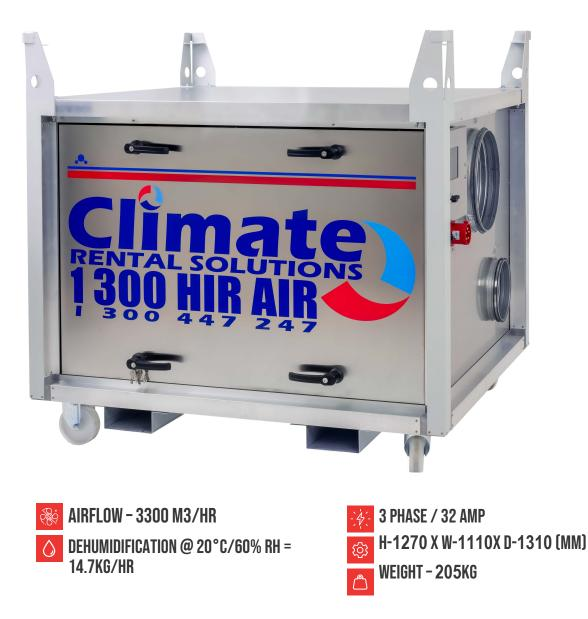
The DT 3300 desiccant dehumidifier is a powerful unit featuring insulated housing with a strong stackable robust frame, fully adjustable EC motor, PTC (Positive Temperature Control) Reactivation heater, Built-in PLC with touch screen, Rotation guard, filter alarm, run-time-meter and service alarm.
